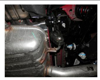
**Step 3.** Working front to rear disengage all welded hangers from the rubber insulators and remove the muffler assembly. (Retain the insulators as they will be needed to mount the new MAGNAFLOW system.) Once the OEM system is on the ground transfer both valve motors over to the new Magnaflow exhaust system using the OEM fasteners.
