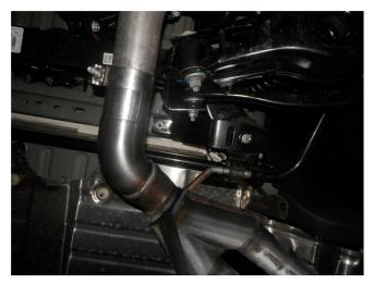
**Step 5.** Install the P/S Tail Pipe Assembly in the same manner. Leave all clamps loose for final adjustment of the system.
