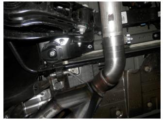
**Step 4.** Begin installation of the new system by sliding the D/S Tail Pipe Assembly inlet onto the cut outlet of the OEM exhaust and loosely fasten with the supplied 2.75" clamp. Fit the hangers into the rubber insulators.
