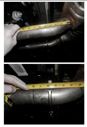
**Step 1.** It is necessary to cut the factory exhaust system to install the new Magnaflow unit. To do this measure 5.75" in front of the welds on the rear muffler inlets. Deburr the cut pipes to facilitate installation of the new system.
